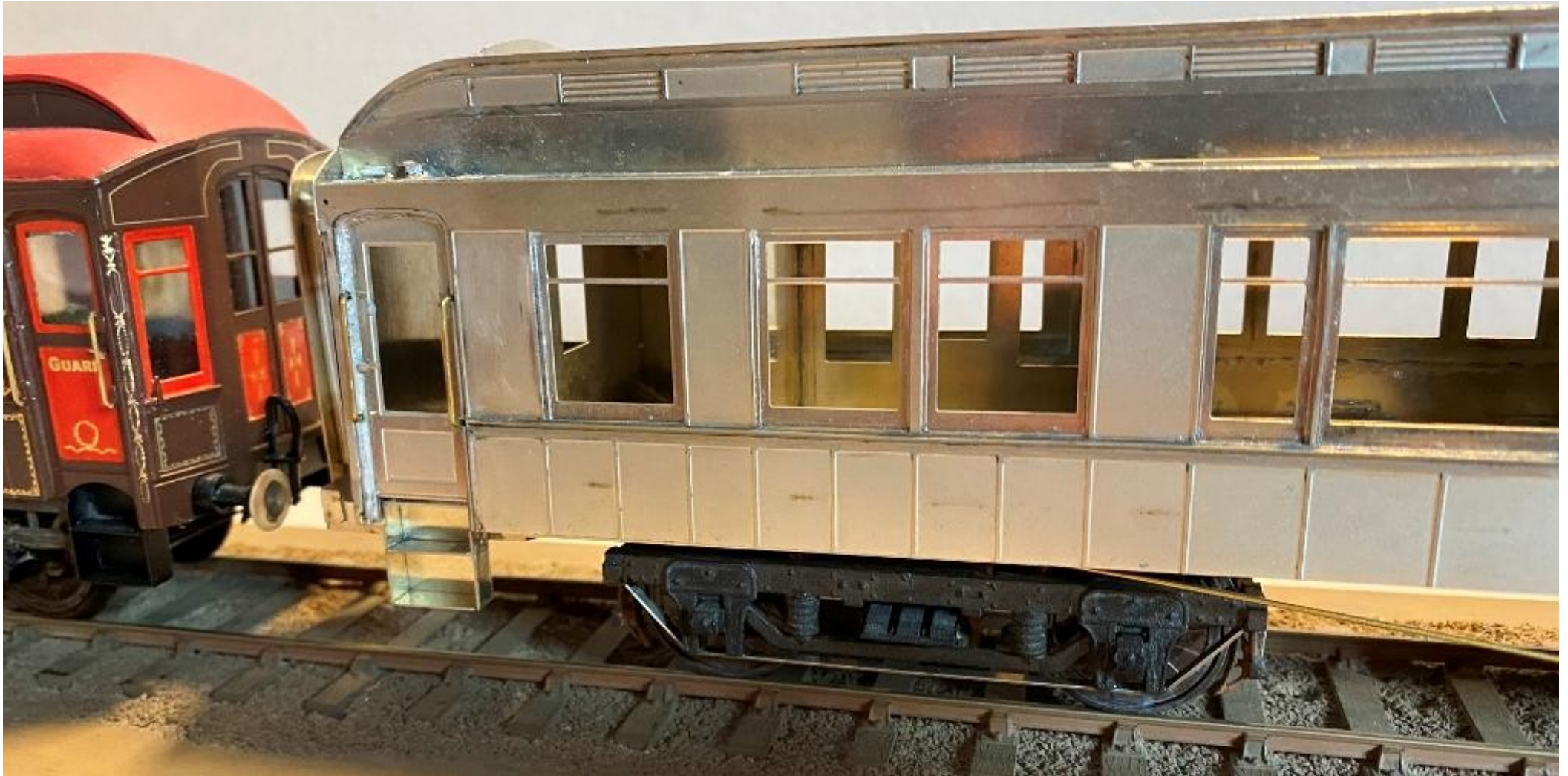
Photo 6: The etched formers for the roof and clerestory have been added. These will be infilled with timber (basswood) and sanded to match the roof profile seen on van no. 29 adjacent. Buffers and a screw coupling have yet to be fitted to the headstock at this end. Within the set the cars will be coupled with MagClic magnetic couplings.
