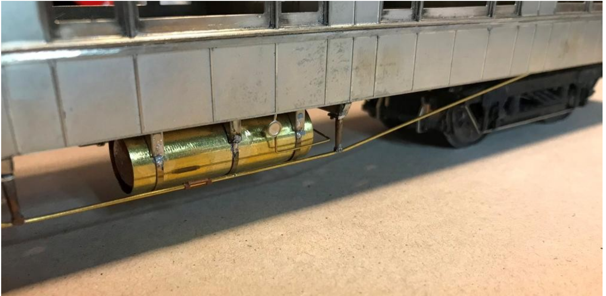
Photo 5: The remaining underfloor detail included cast brass queen posts, brass truss rods with moulded plastic turnbuckles from EDM Models and gas tanks from brass tube. Although the train was illuminated with electric lights powered by the dynamo in van no. 29, supplementary gas lighting was also provided; later in life 'Her Majesty' was altered to run as a 'loose' car and had to rely solely on gas lighting.
