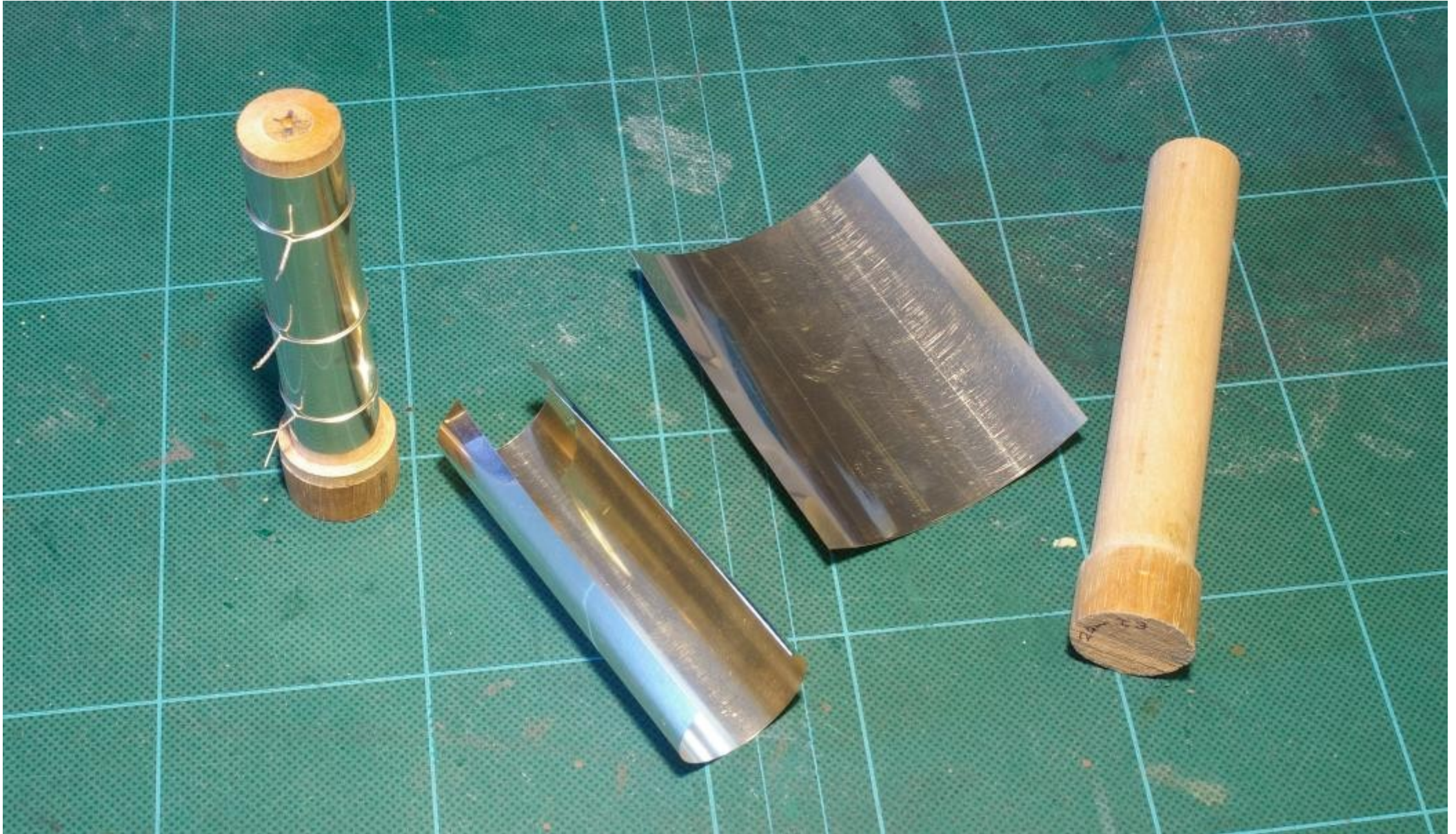
The boiler wrapped around a former, ready to be soldered along the seam
