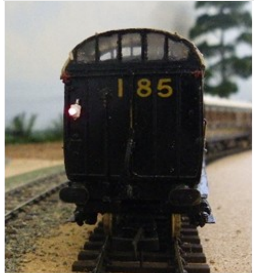
Bogies fitted running both interior lights and tail lamp
