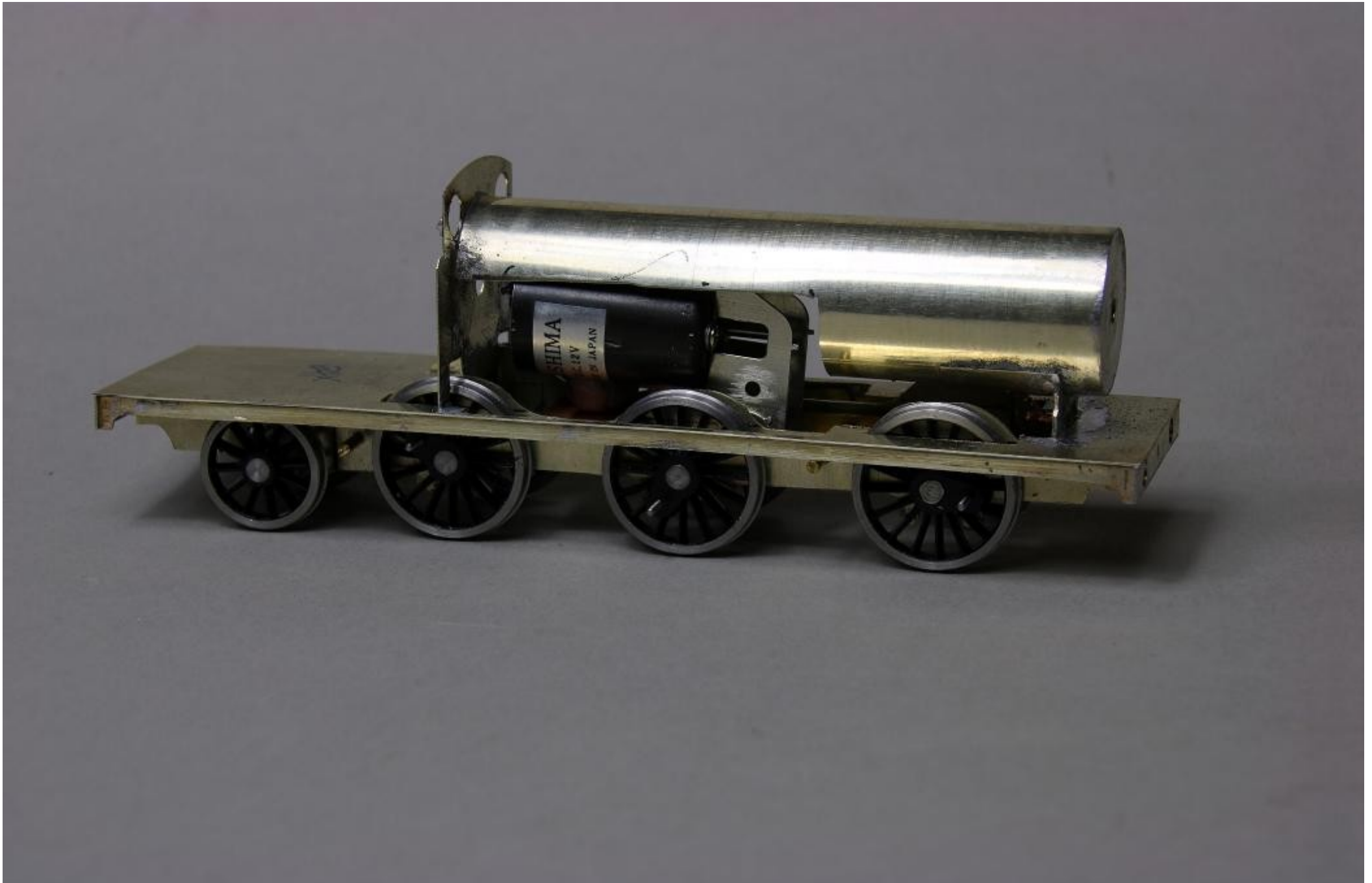
The motor/gearbox fitted to the chassis and checked for clearance
