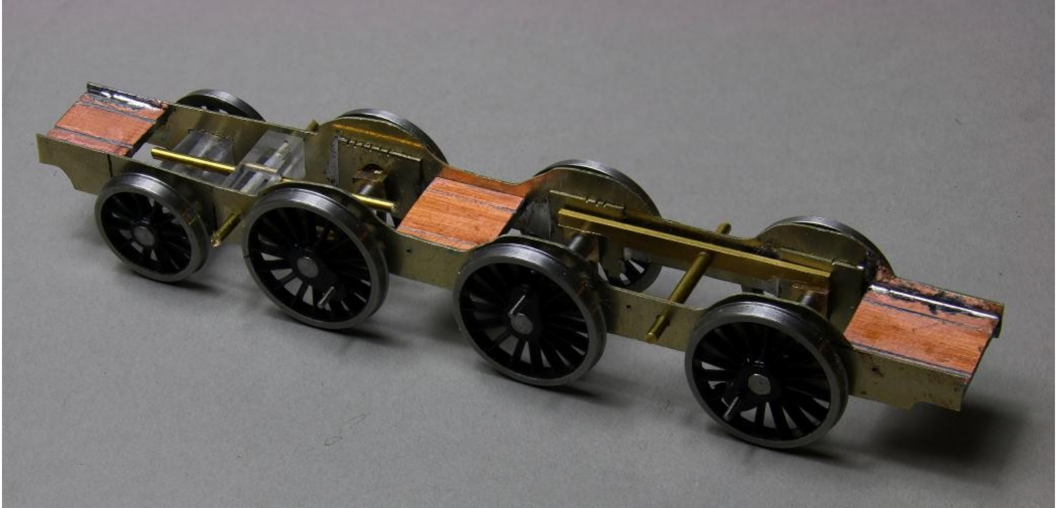
The rolling chassis, showing the twin side beams at the front, single central beam at the rear, and radial axle box for the trailing wheels
