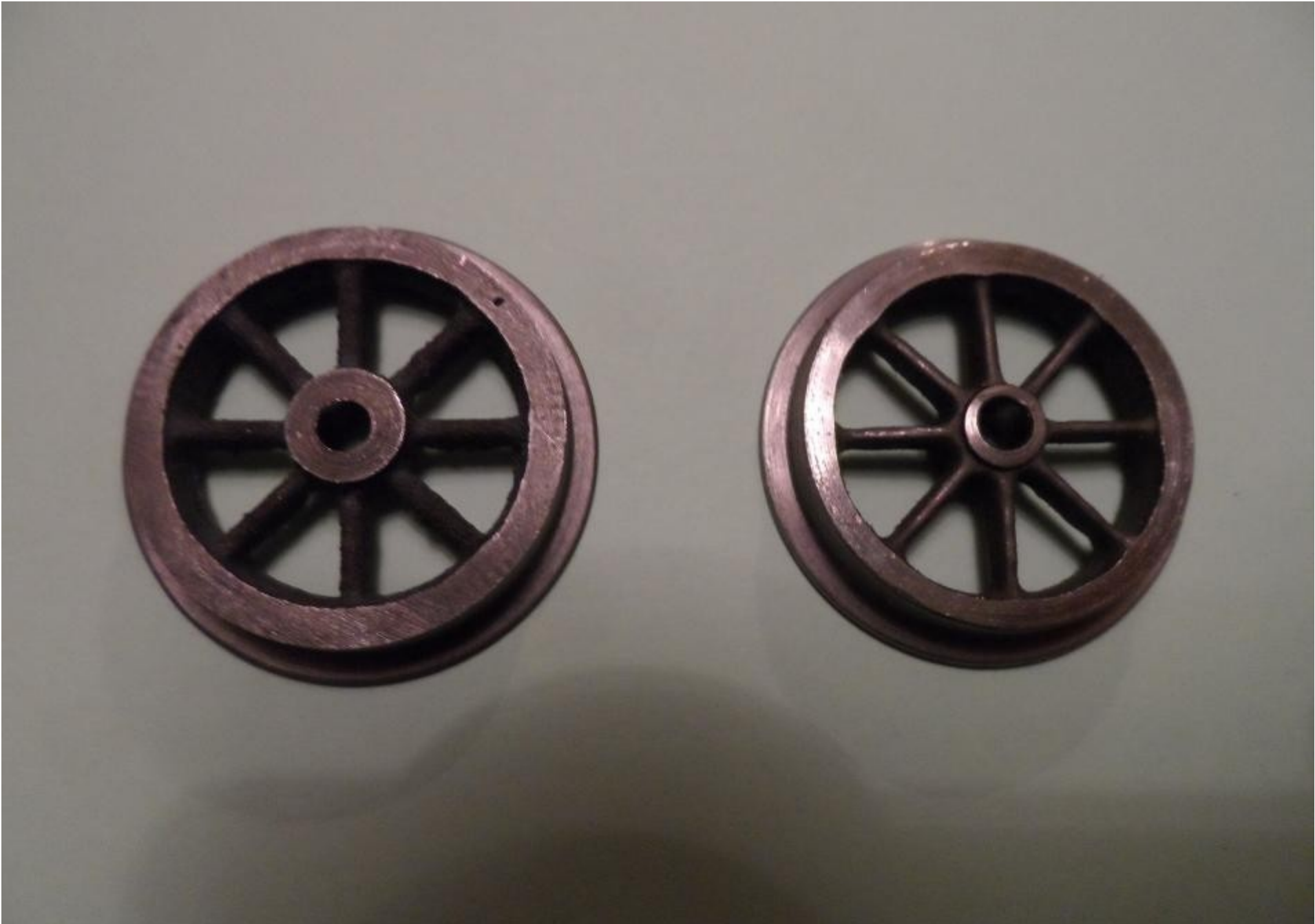
The contrast between a sand cast and a lost wax cast wheel.
