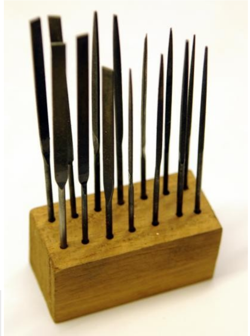
Picture 64 A selection of needle files in a storage block. Flat, round, half round, square and three square in a range of different grades.
