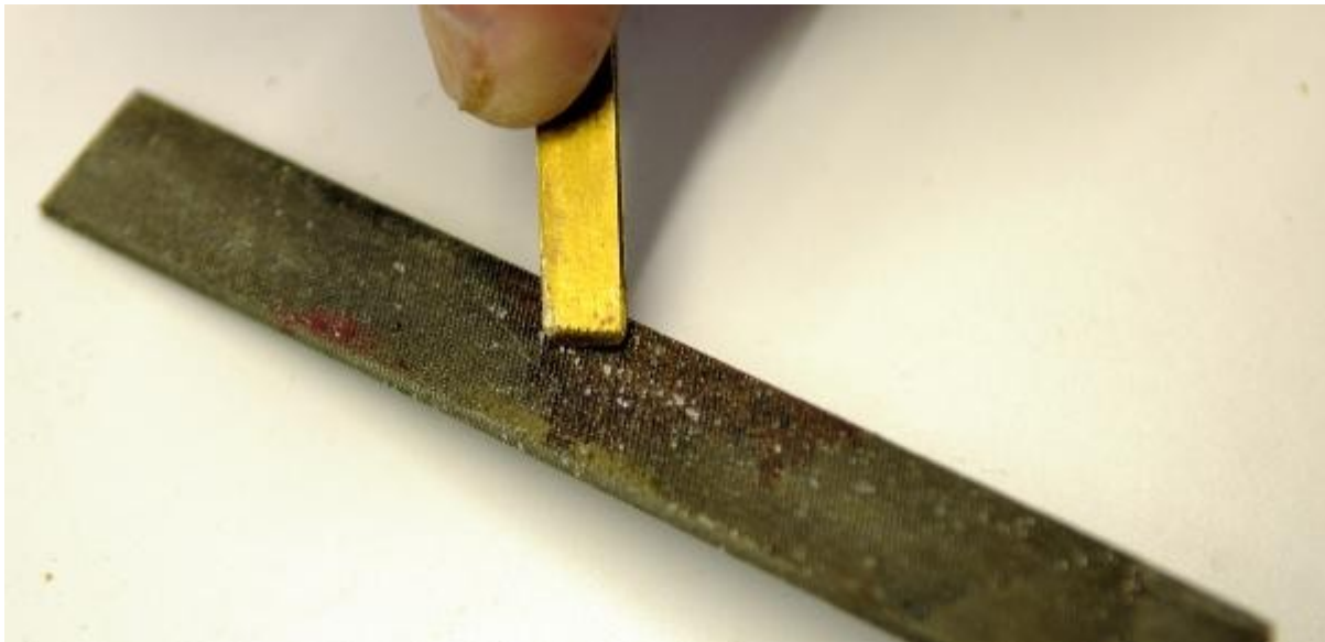
Picture 61 Cleaning a clogged file by pushing a piece of brass across the file.
