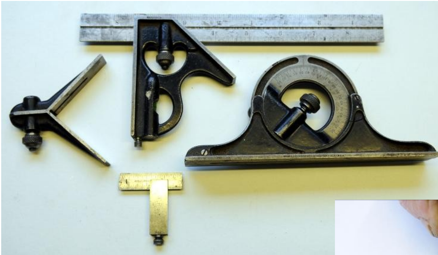
Picture 26 Large adjustable try square as part of a combination set. A small adjustable try square is shown below..
