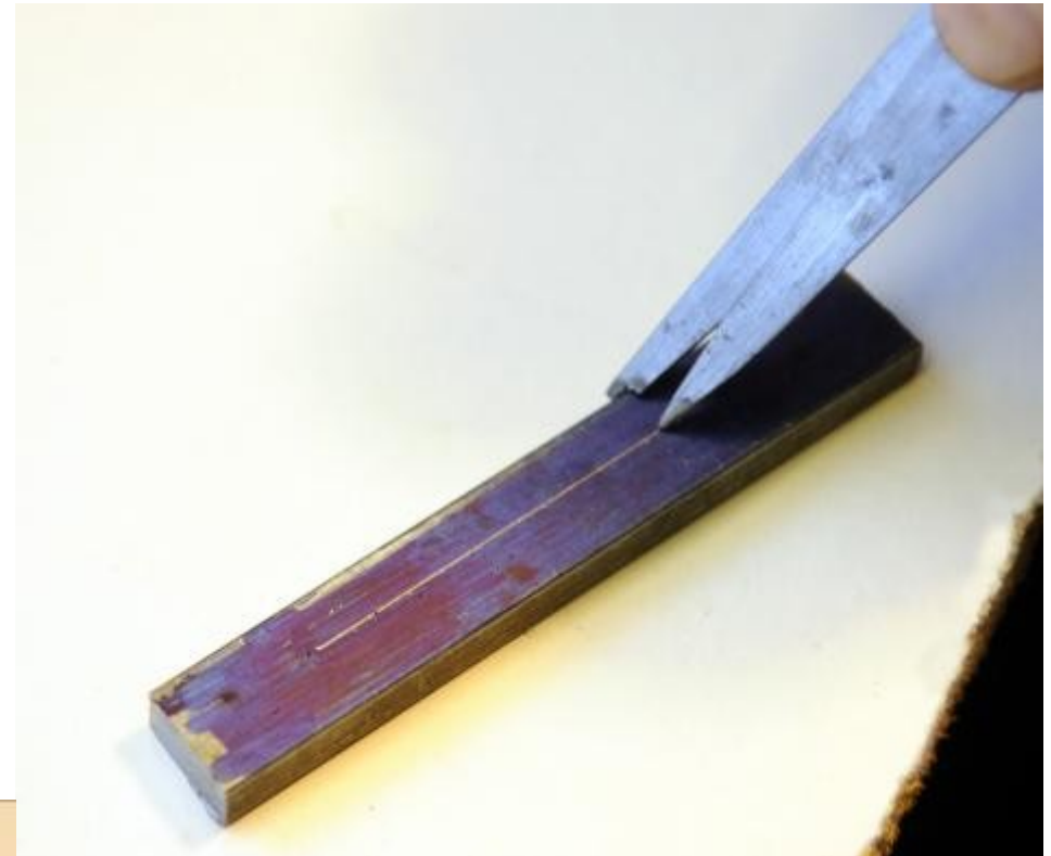
Picture 24 Scribing a line parallel to an edge using odd leg callipers.
