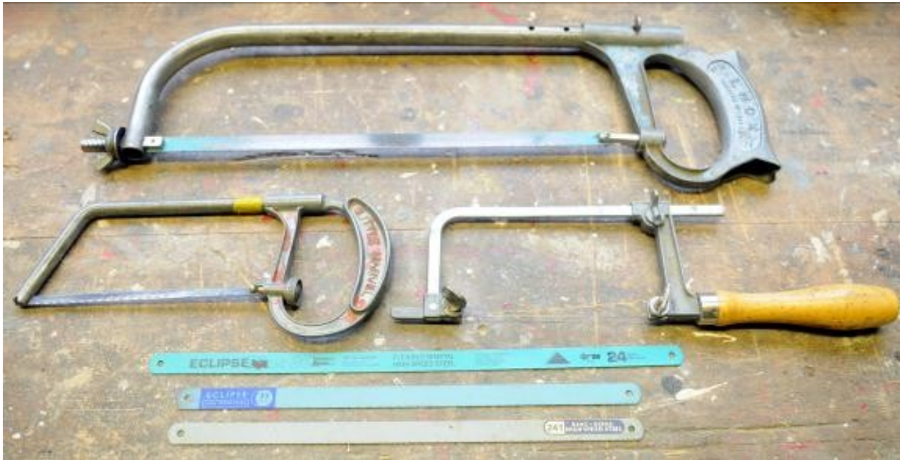
Picture 31 Saws for metal. The top hacksaw blade is a 12 inch long bi-metal blade with 24 teeth per inch. The middle one is a 10 inch blade with 32 teeth per inch whilst the bottom one is a 10 inch blade with 24 teeth per inch.
