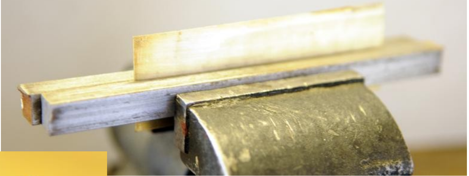
Picture 66 bending sheet metal using two lengths of square bar.
