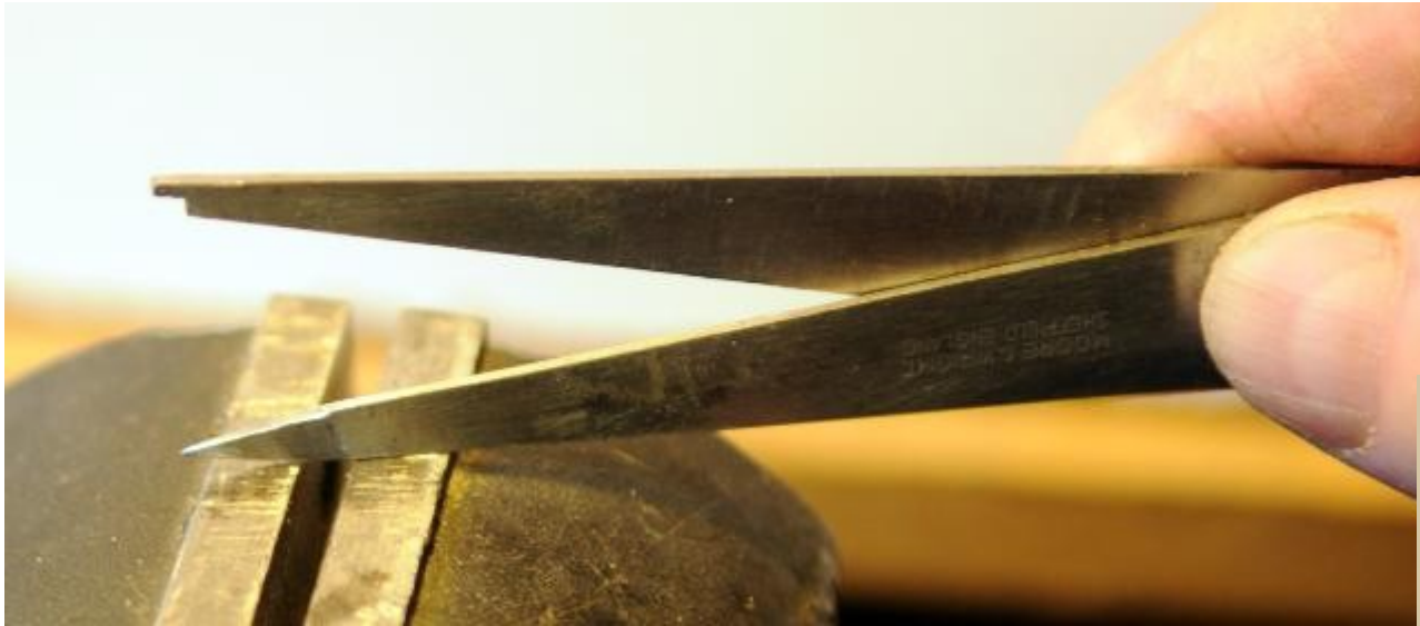
Picture 22 Setting odd leg callipers to size by tapping on the top of the vice
