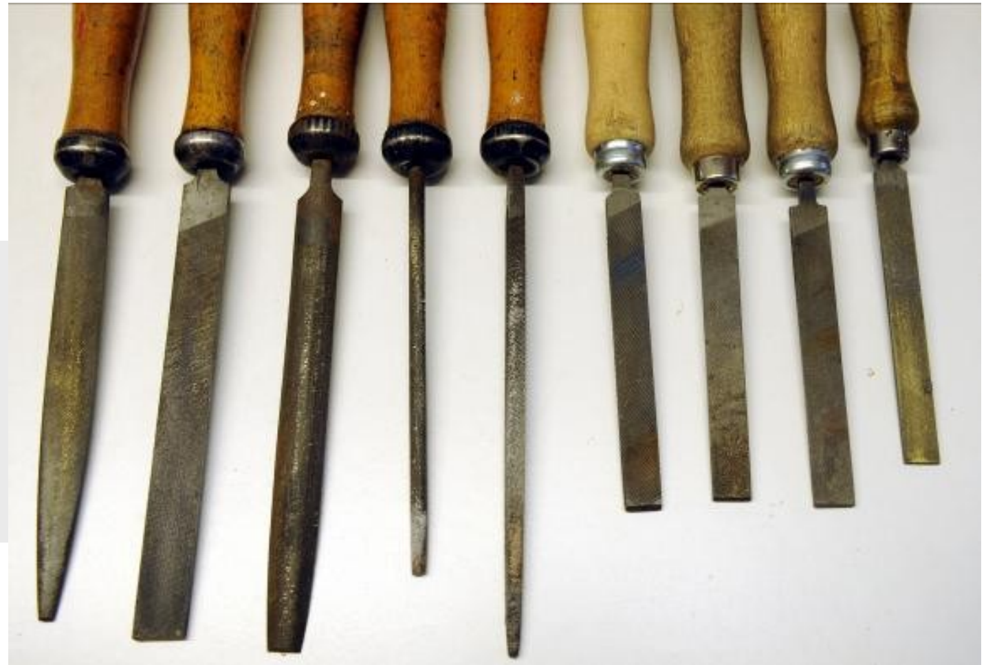
Picture 62 A range of files that will cope with most model making in the smaller scales. From the left crossing, hand, half round, round and square files six inches long and four hand files all four inches long.
