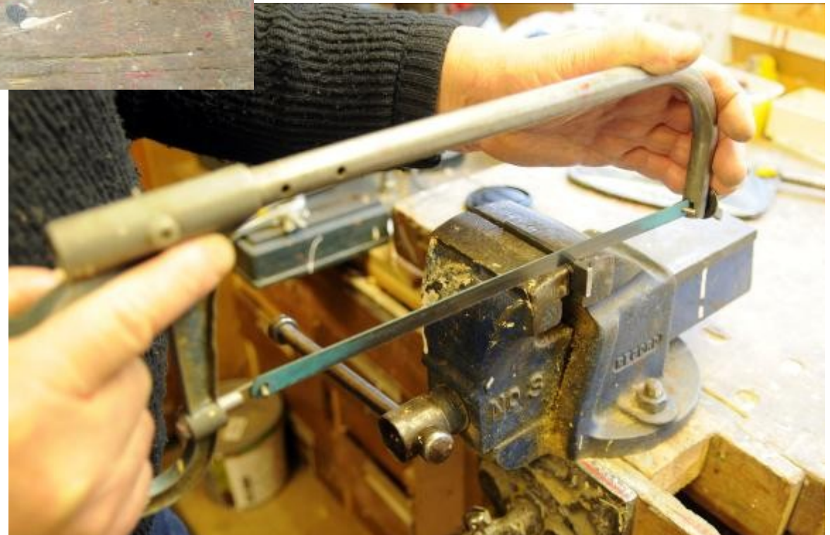
Picture 32 Using the hacksaw. Placing the forefinger of the right hand as shown helps to give a straighter cut. Those who are left handed will need to reverse the hands.
