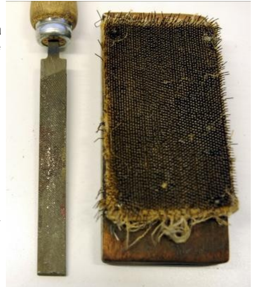
Picture 60 Clogged file and file cleaning brush.
