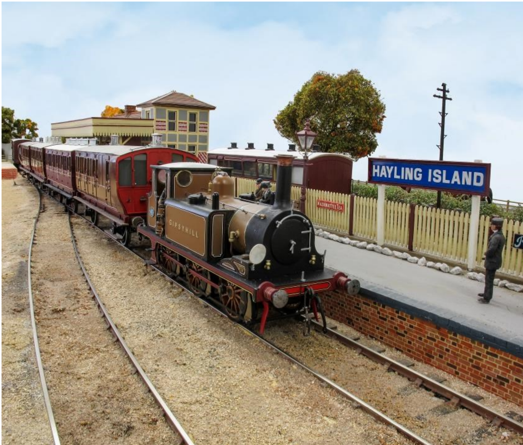
"Gipsyhill" awaiting departure from the terminus. The typical branch set consisted of a Brake Third, a Third, a Composite and a Passenger Brake Van, all still oil lit.
