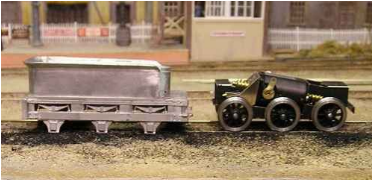
LongRider power bogie, with the extra axle fitted, sitting next to the tender body.
