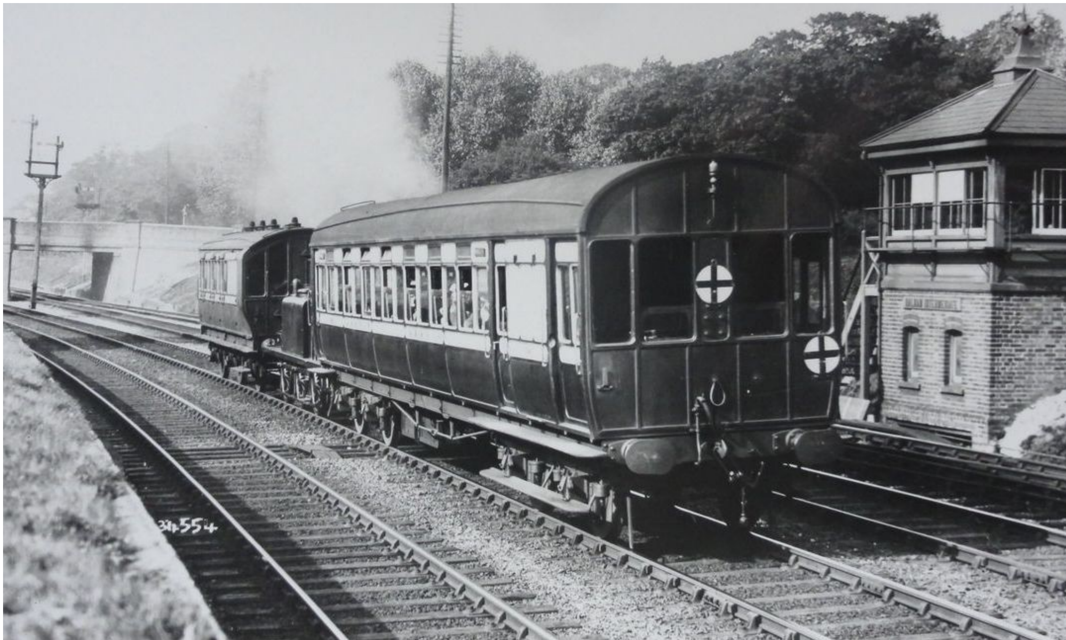
An unknown Terrier passing Balham Intermediate signal box, the balloon coach leading, with a six-wheel brake third behind the engine.
