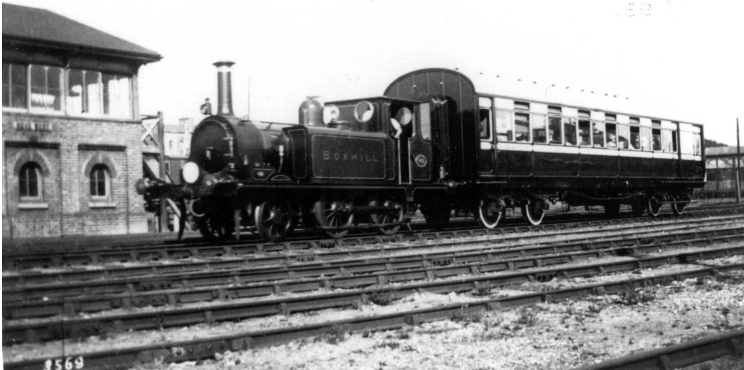
Boxhill as a 2-4-0T, and one of the original trailers, with the unused gangway connection visible, at Hove
