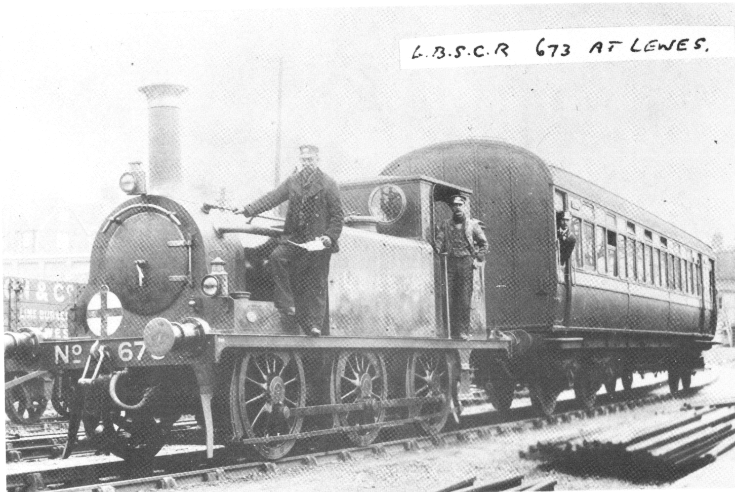
Terrier 673 (formerly Deptford) at Lewes, before conversion to A1X in 1912, coupled to one of the later Balloon autotrailers.
