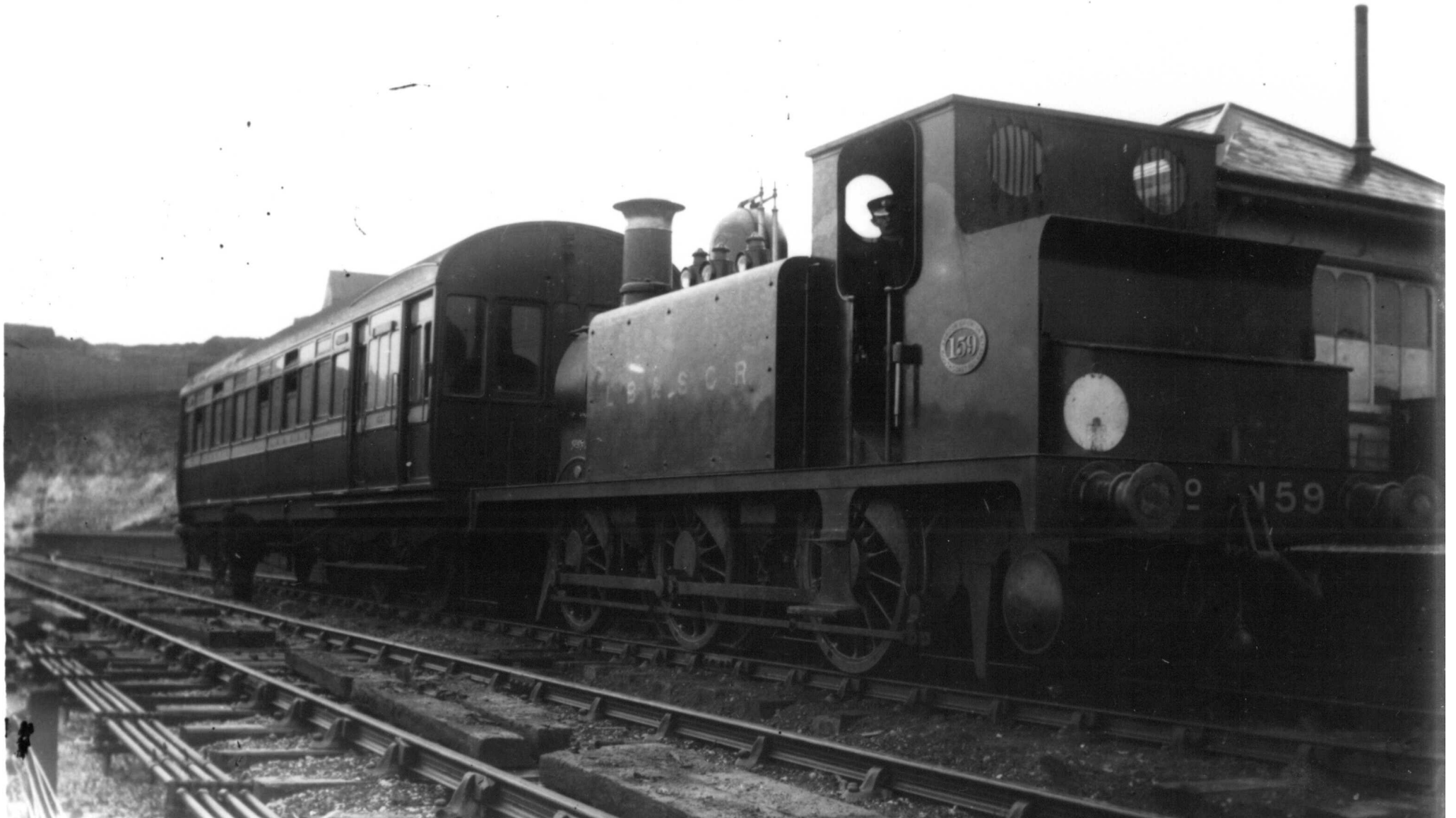
It is hard to think of a more inappropriate combination! A non-P/P-fitted goods loco combined with a balloon autococh, the wrong way round, at Dyke Station. Note the single line staff actually displayed in the holder fixed to the cabside. Probably, the only photo that shows this fixture being correctly used.
