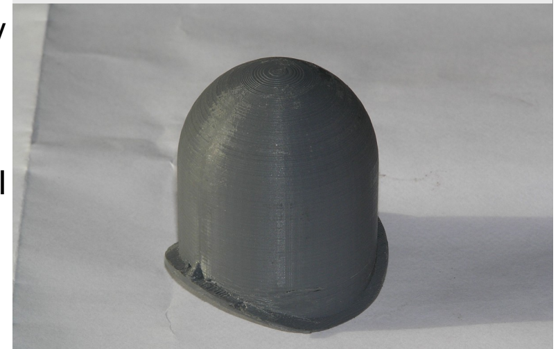
The First Grey Printed Dome (from Sketchup) after trimming
