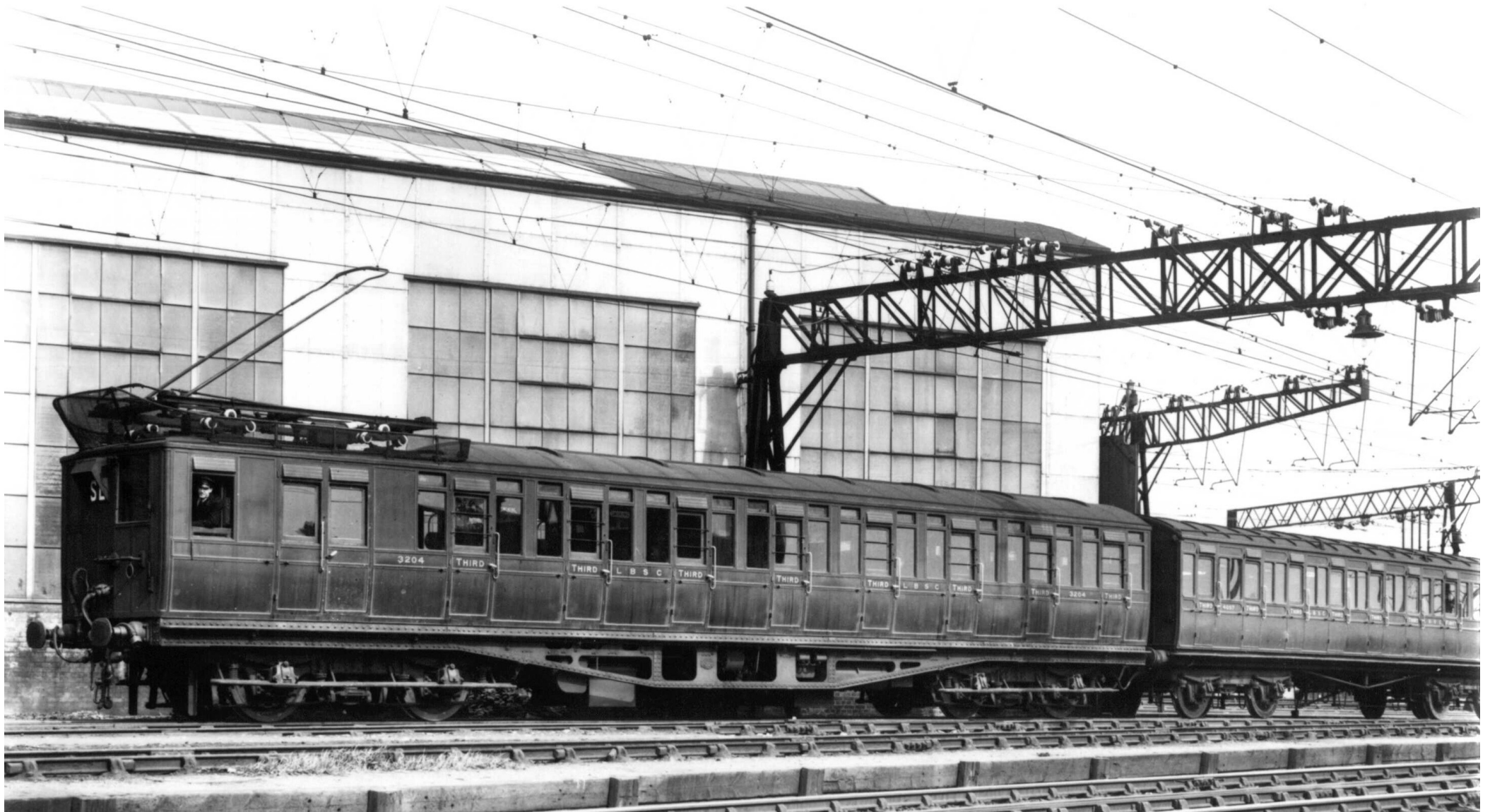
The later 2 carriage South London set at Peckham Rye depot. The visual differences between the two vehicles are evident. Square panelling, heavy trussed underframe and greater width and height of the original motor unit, compared with the “traditional” Brighton styling, dating back to the 1890’s, of the new trailer.
