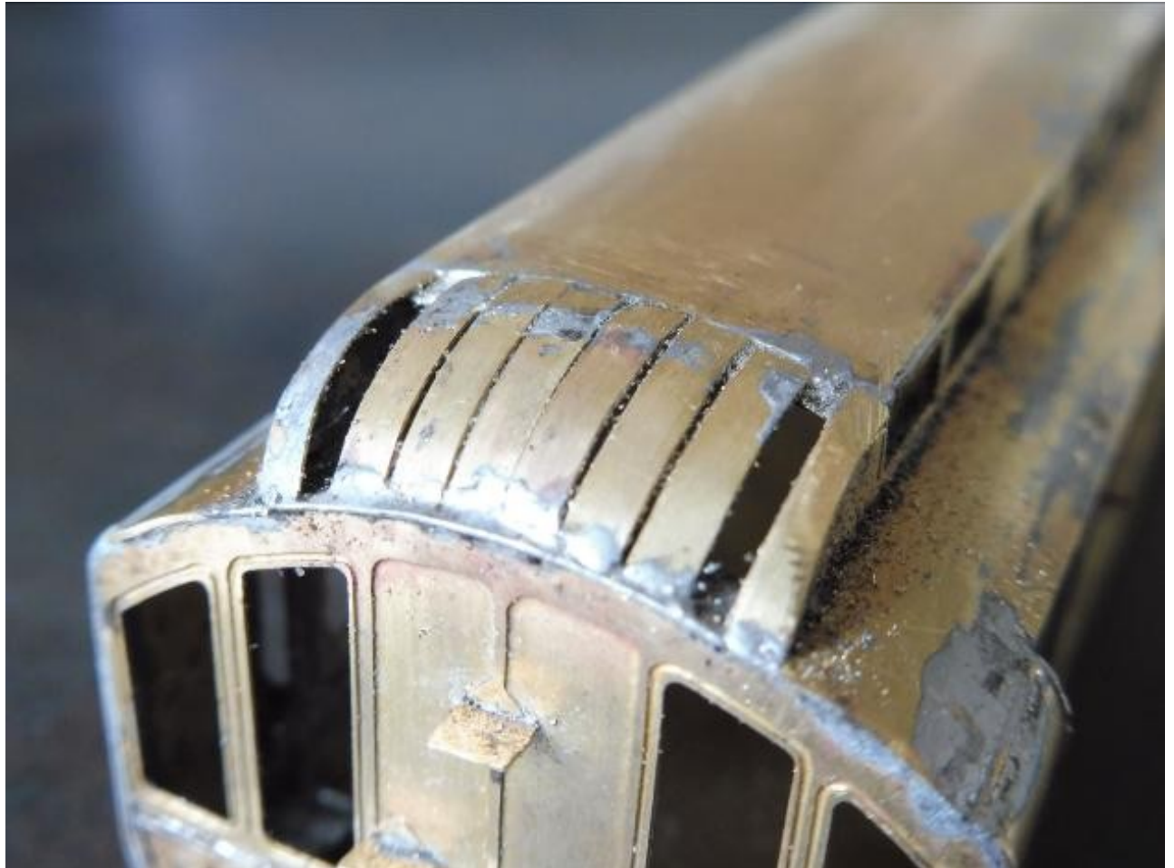
Most strips attached, ready for the last two, before filling.
