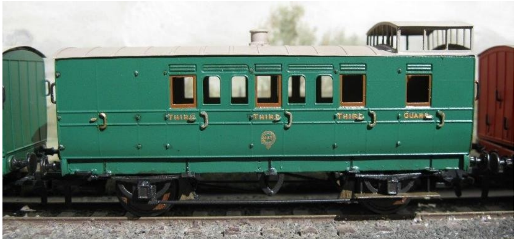
Type 15G brake luggage third with one full compartment and two coupés
