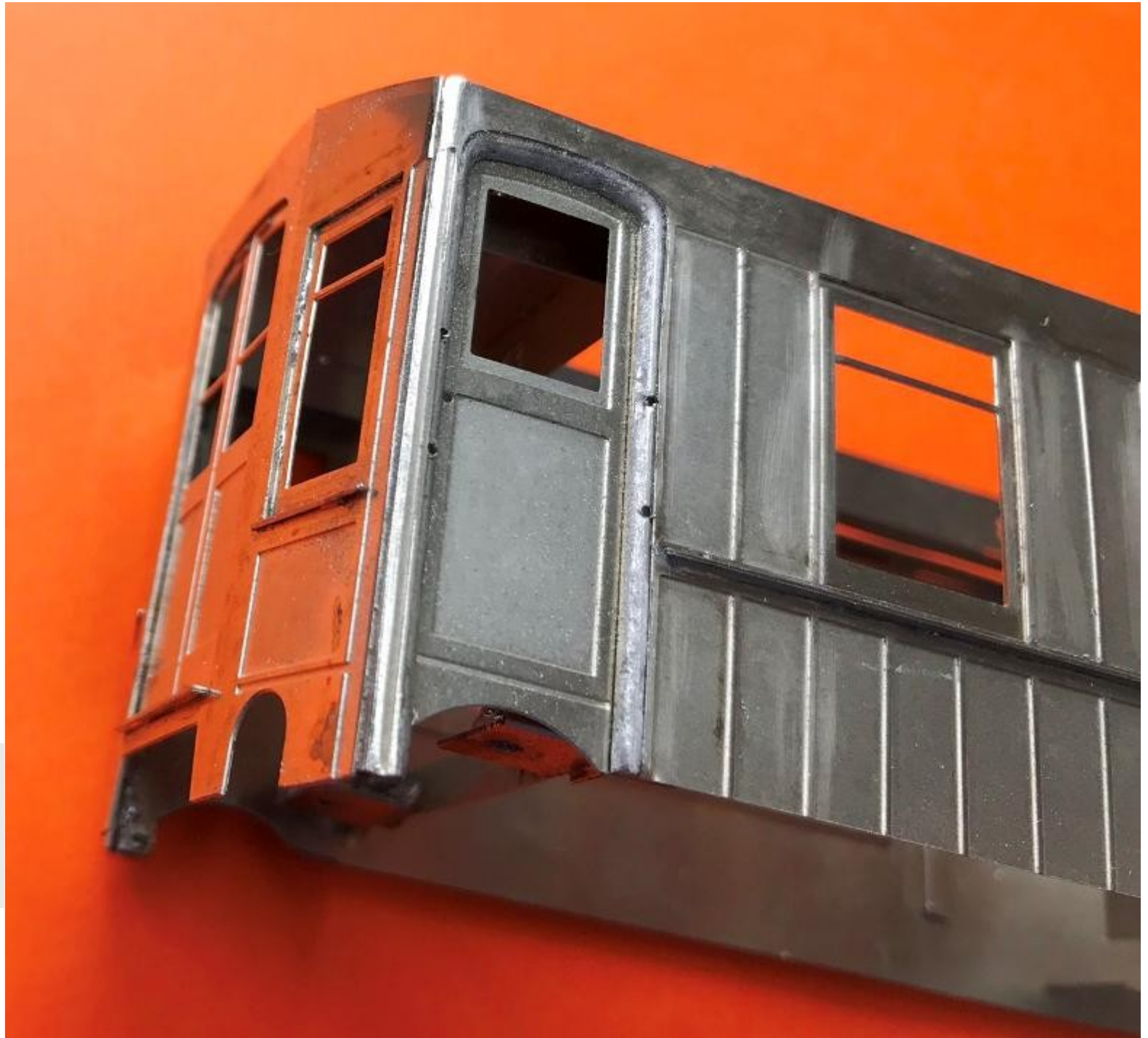
Photo 10: Adding the ends to the carriage body (Peter Warren)
