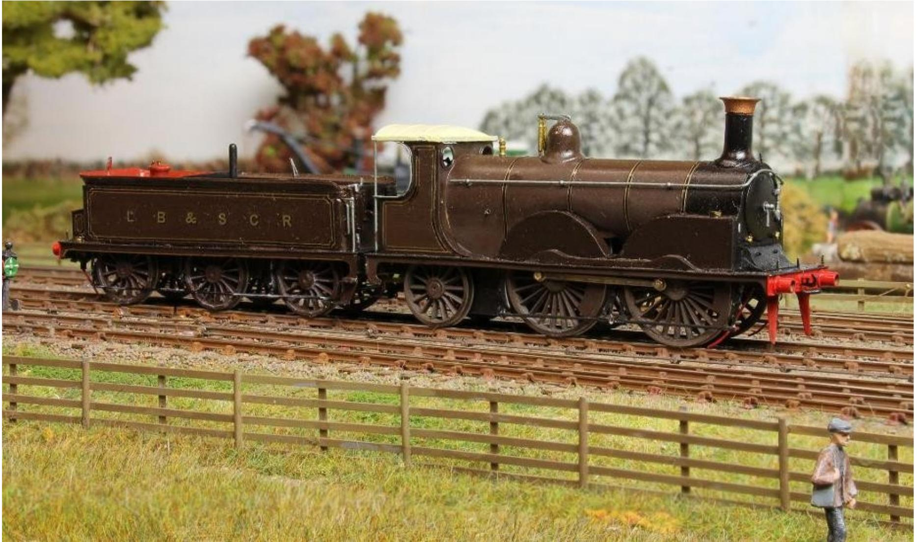
I2 Scratchbuilt using a Mashima motor, High Level gearbox, Sharman bogie and pony wheels and Gibson drivers. It is fully compensated with split axle pick up, Perspex radial axle box and simple bogie pivot. The painting process has been the same as for the E4x but the panels were lined directly using precision lining gold. The upper panels had to be redone using transfers. Painting involved a coat of gloss
