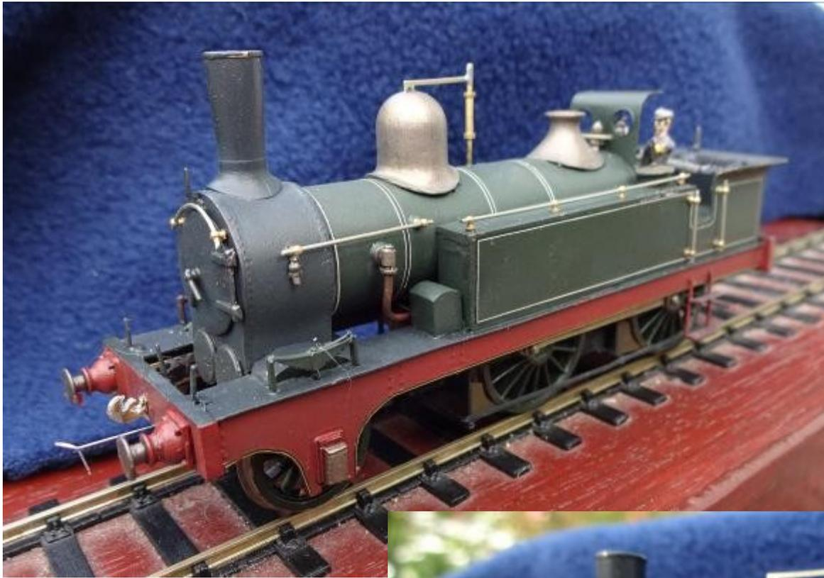
Finally, with crew (the thinnest ones that I could find) on board and the masking fluid removed from the tyres! Less visible are the lumps of lead in the boiler and sidetanks.
