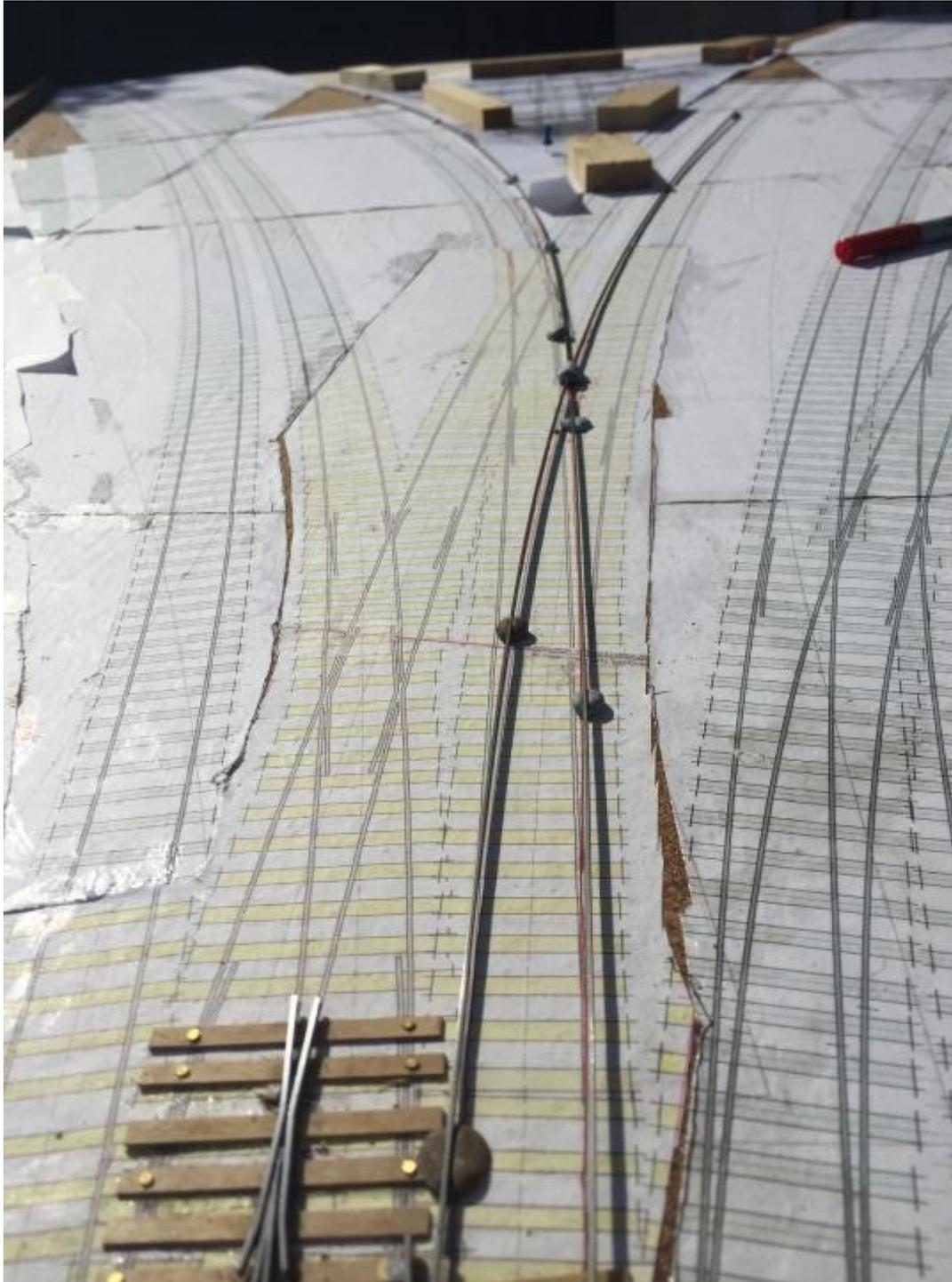
Figure 19 Some alignment adjustments into the station – there's no substitute for rail and Blu-tack!
