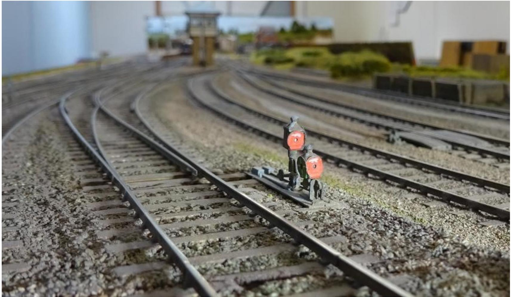
hand one reading across the main lines towards the station. The last two (above), numbers 17 and 18 are close to the edge of the embankment so are mounted one behind the other. The higher one at the back is for the left hand route and the lower one to the right into the goods yard. I have seen a photograph of a stack of three discs at East Croydon.
