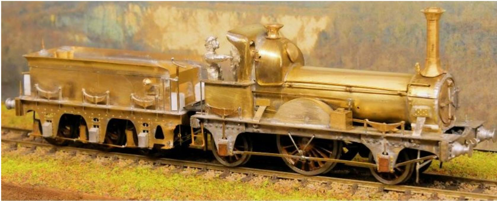
*Figure 6. The model of Seaford ready for the “paint shop”, posed on a shallow diorama depicting a North Downs scene (Riddlesdown Quarry, Warlingham), with a trial fit of some of the small components that will be properly attached after painting.*
