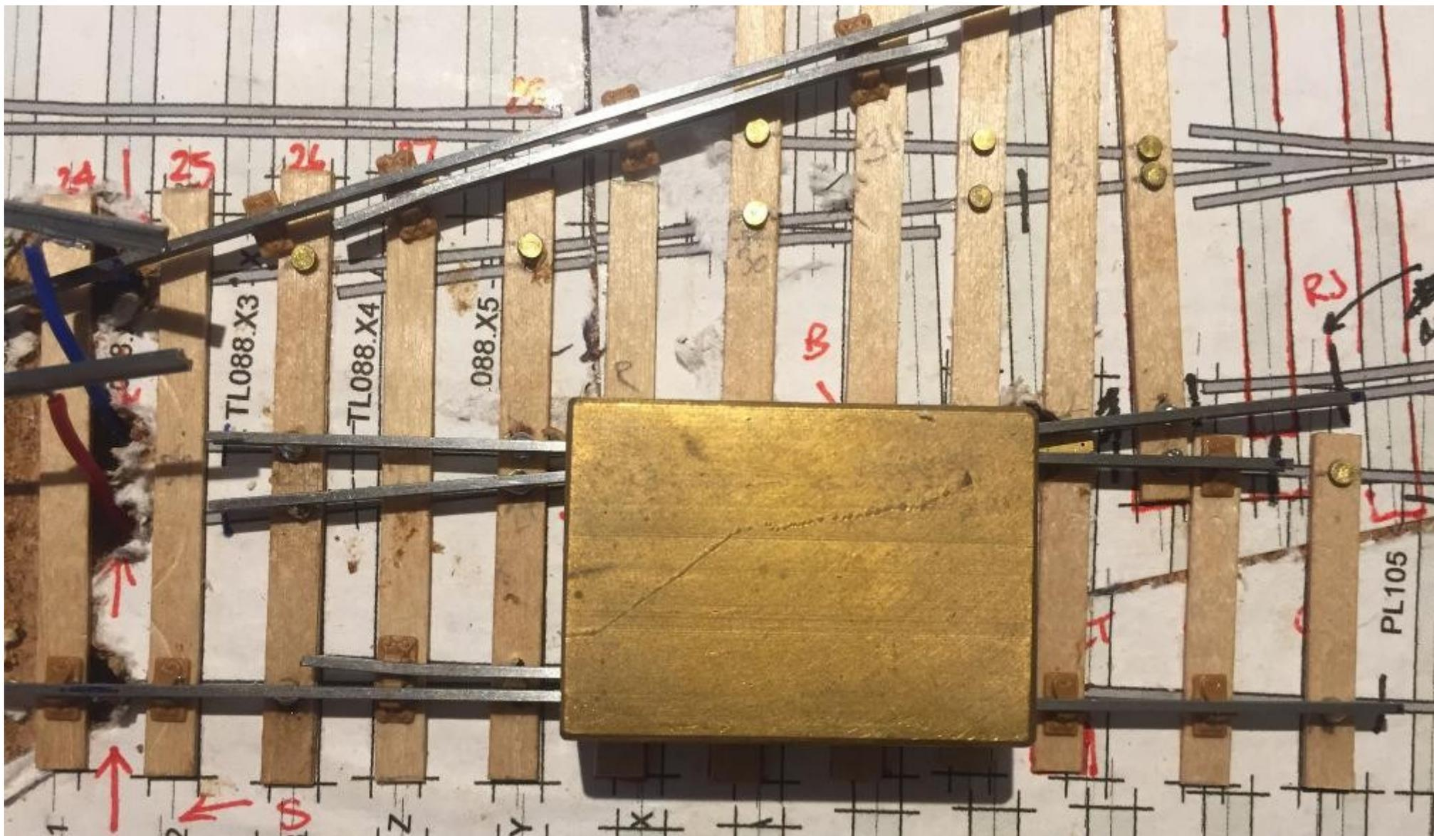
Figure 8 Stock rail and crossing fitted. Conventional gauges are fine for construction, but there's nothing like a mint gauge for that 'smoothness' check! Plastic chairs are not yet glued, in fact I won't be gluing any of them until I have had a proper operational test, just in case I need to make any slight adjustments in alignment.
