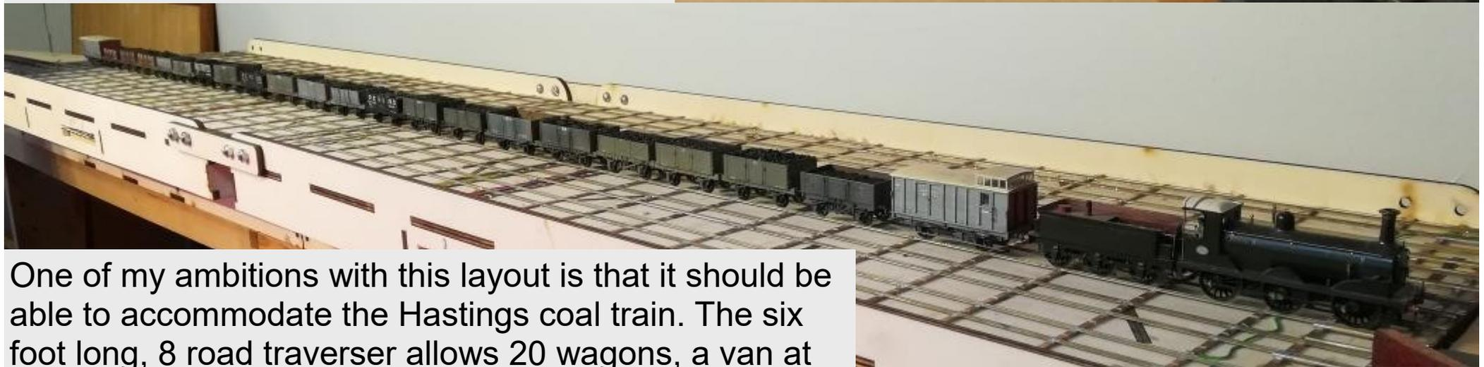
One of my ambitions with this layout is that it should be able to accommodate the Hastings coal train. The six foot long, 8 road traverser allows 20 wagons, a van at each end and a loco, although it is a snug fit.
