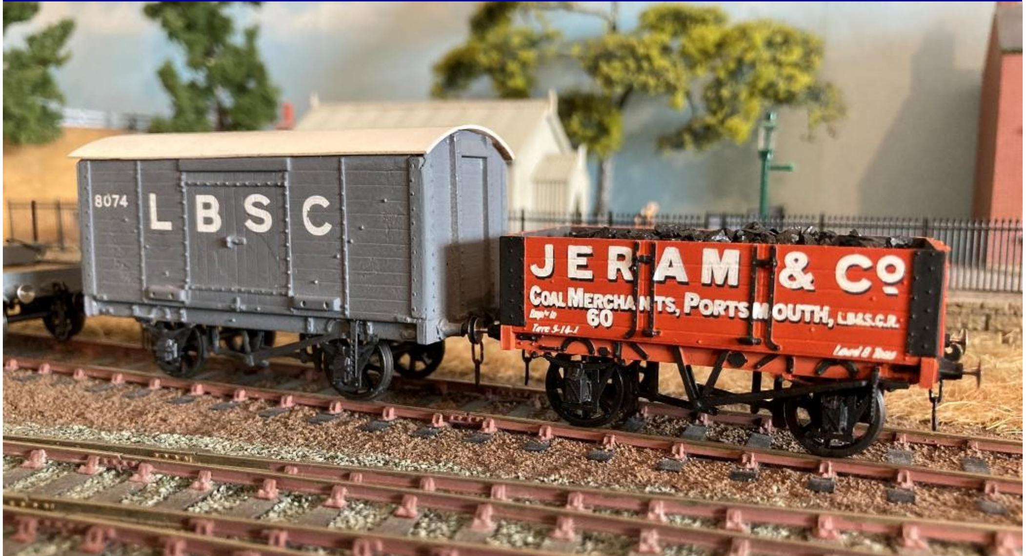
The covered van is from a NuCast kit with Alan Gibson P4 wheels. I got it already assembled, but in need of some renovation and, although it is not compensated, it is squarely built and quite heavy, so track holding doesn't seem to be a issue. It is fitted with single V hanger single side brakes and a spare metal brake lever from a Hornby PO wagon.
