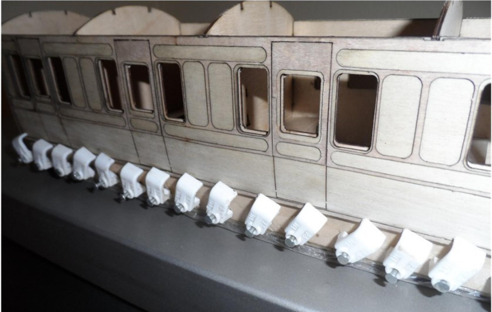
You can see that I have just carefully re-applied pressure along the bottom strip of the fret with the cable clamps. They are just carefully pushed down. Hopefully the bottom strip will not distort as I have made them slightly thicker so they can be sanded back to the under surface of the floor. But please check that it is dead straight as you apply pressure from the cable clips.
