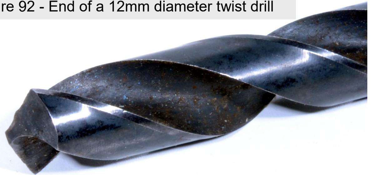
Picture 93 Parts of a twist drill
