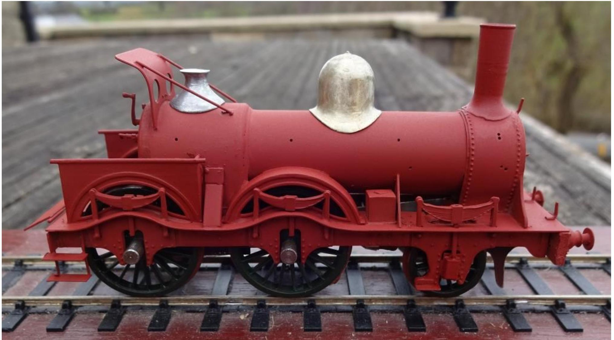
The stovepipe chimney is one of Ian MacCormac's prints. The original print is very fine and commendably thin, but caused me to worry about vulnerability. I therefore ran a coat of Araldite down the inside to give it a bit more substance, without affecting the top rim too much.
