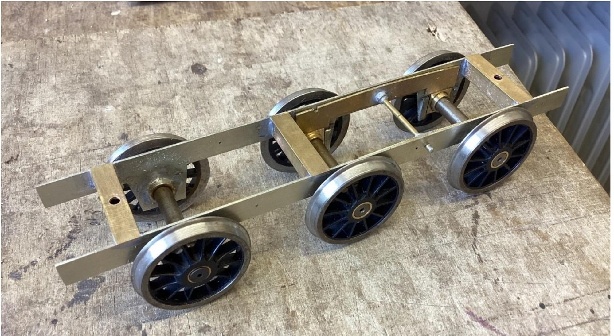
The basic frame, soldered (Carrs Speedy Solder) together, using my own  $\frac{1}{4}$ " square brass frame spacers. Each one has a lip on top, that fitted into the filed slots as shown in the previous photo. The double beams were cut out from scrap brass, and pivoted in the centre via  $\frac{1}{16}$ " brass tubing, with a 0.8mm n/s pin. Each one rests on top of the hornblocks as per the locomotive. Minute amounts of careful filing of the bottom of the beams result in a horizontal chassis.
