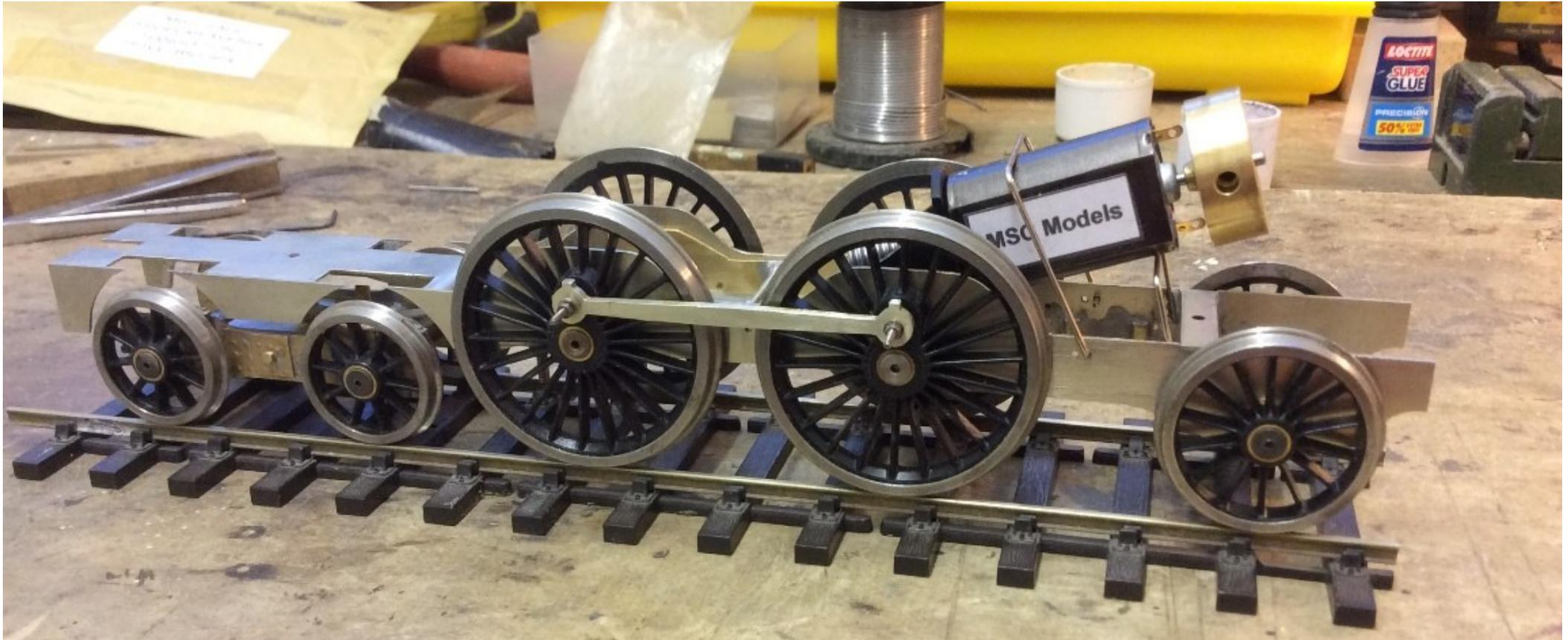
This view shows a near complete chassis after it has been fitted with the excellent MSC Models SM motor with 30:1 single reduction gearbox ([www.mscmodels.co.uk](http://www.mscmodels.co.uk)) with flywheel and run-in in both directions. A double reduction gearbox would have been preferable but it wouldn't fit in. The single reduction gearbox still gives superb control.
