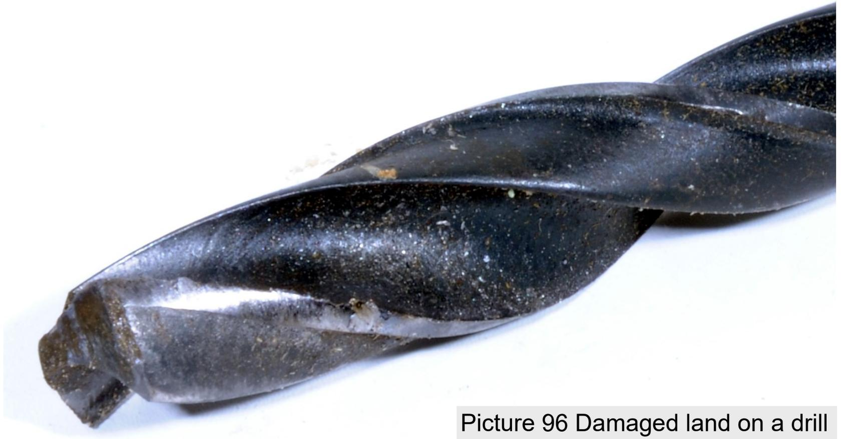
Picture 96 Damaged land on a drill
