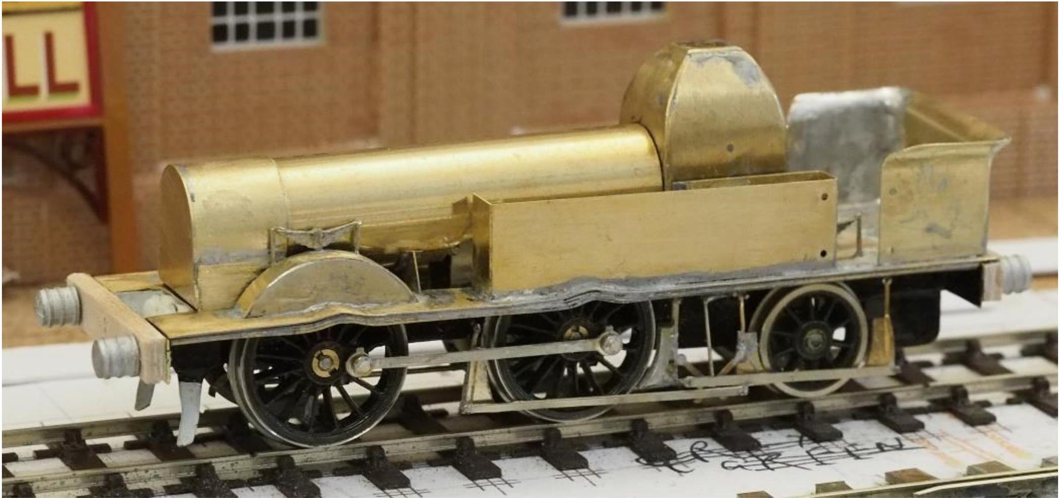
Second test assembly to check the fit of the smokebox and boiler assembly over the motor. Note that the buffer beams (made from layers of a wooden coffee stirring stick) were fitted to the chassis rather than the footplate. The rear half of each side tank and the front half of the boiler assembly were lead filled.
