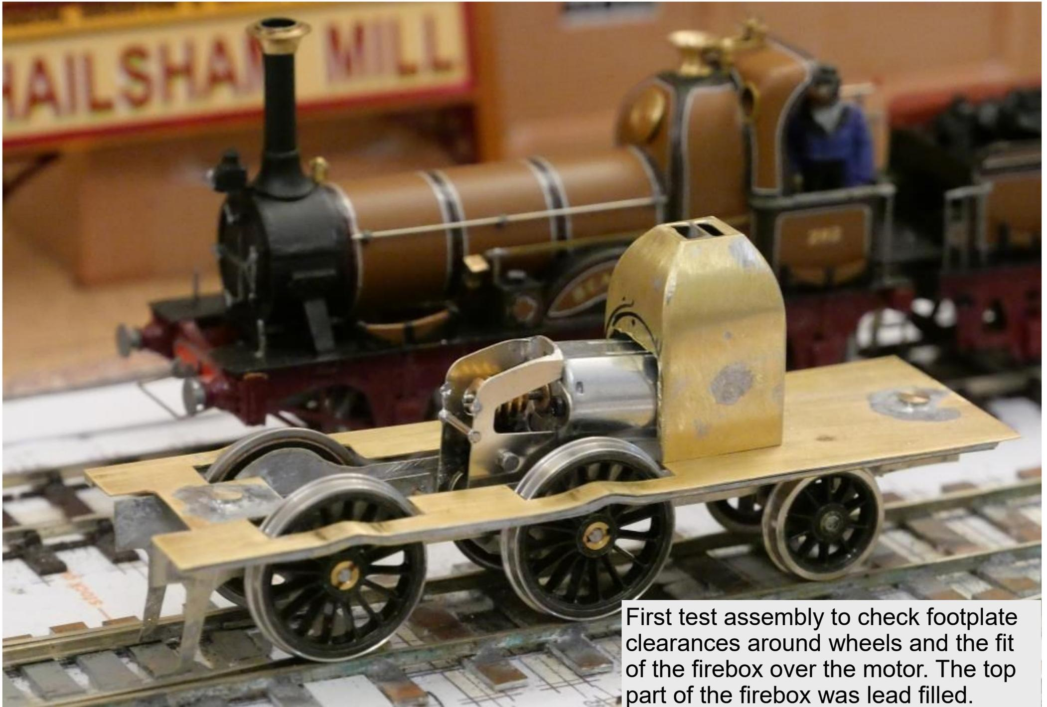
First test assembly to check footplate clearances around wheels and the fit of the firebox over the motor. The top part of the firebox was lead filled.
