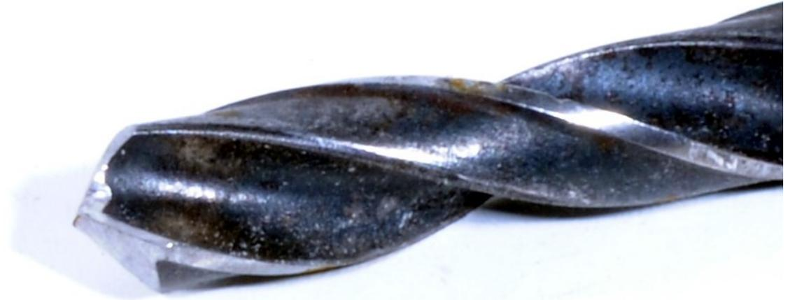
Picture 105 Modified rake angle
