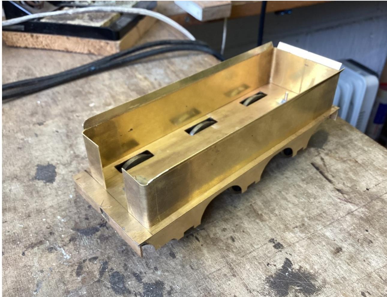
Before any brass was cut, cardboard footplate templates were again used. The most critical area was giving enough clearance for the middle and rear axles to move up within the slots. The two sideframes were then cut out and soldered in place.
