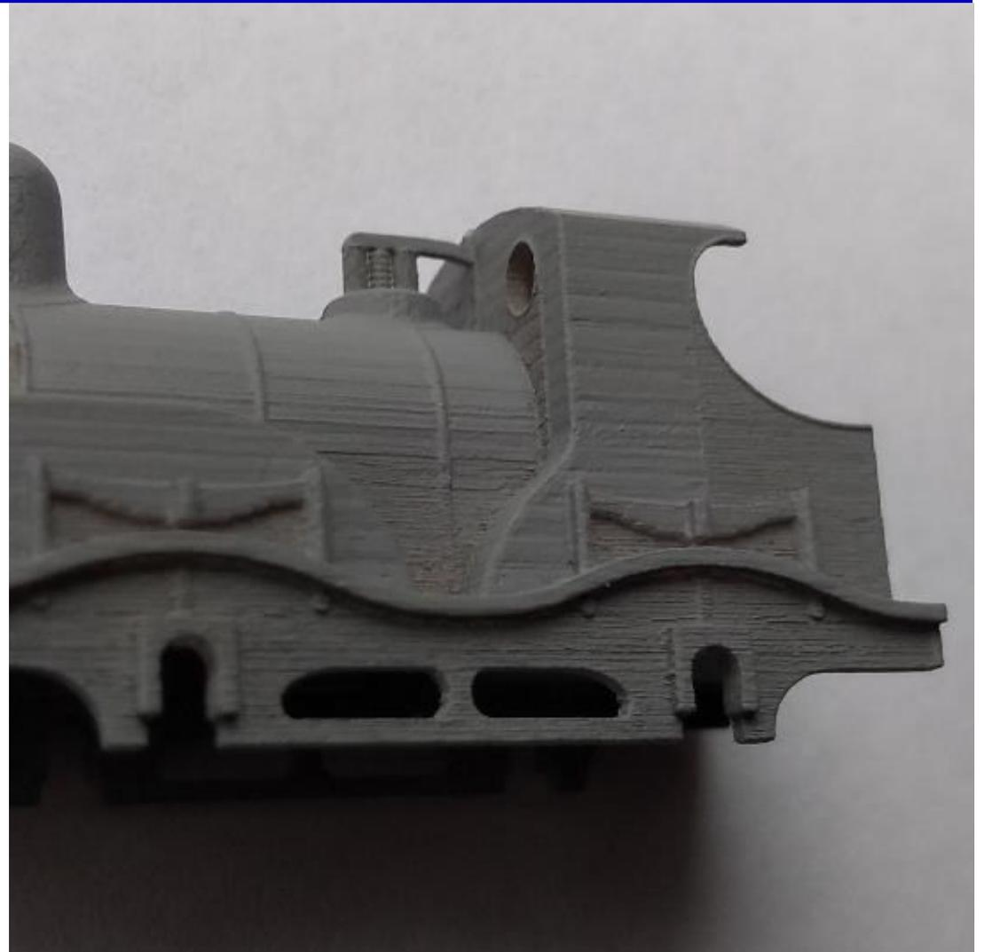
Most dimensions were very close but a lot of detail needed to go, which sanding was going to remove anyway. I removed the springs, boiler bands, dome, safety valve, smokebox door, cab roof and a portion of the outside frames. A new roof, reshaped cabsides, new dome, safety valve, footsteps, front wing plates and smokebox door were added.
