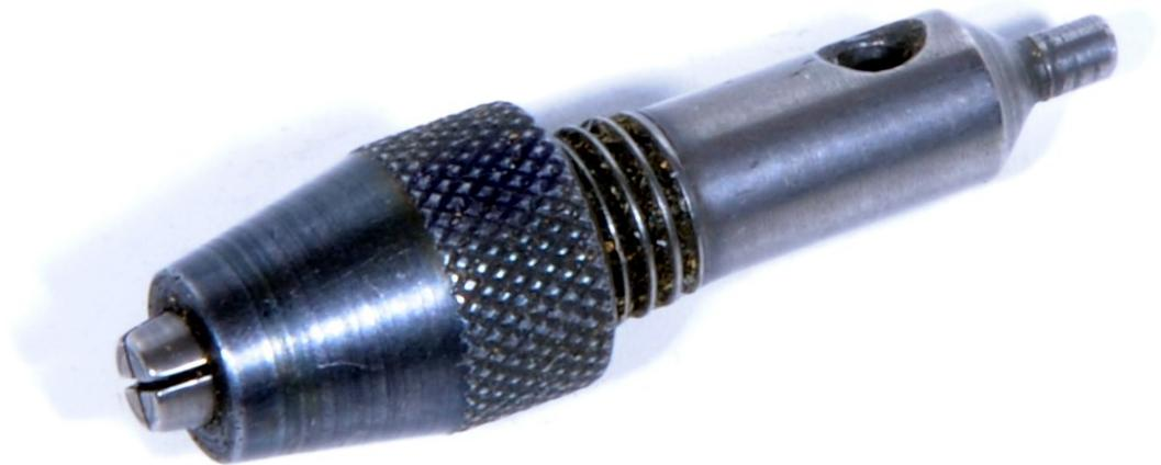
Picture 103 Modified pin chuck
