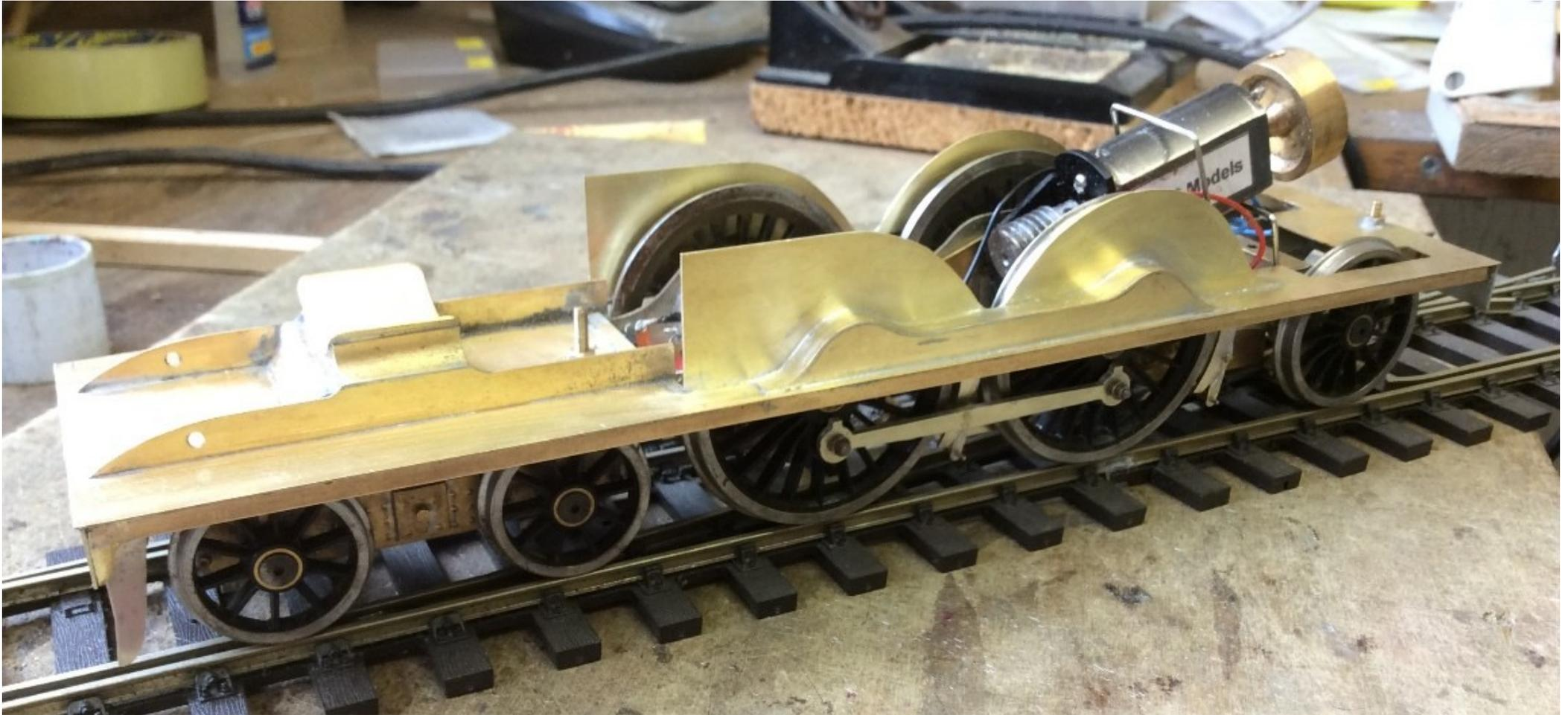
The footplate has now had side valancing (3mm x 3mm L angle) fitted, along with the headstocks, saddle sideframes, curved saddle, and guard irons, as per the drawing. Because all four drivers and coupling rods move up and down, the radii of both splashers had to be increased slightly for the maximum upward movement. Again, these areas are subtle and not noticeable. Just visible behind the rear driver is a brake hanger and shoe.
