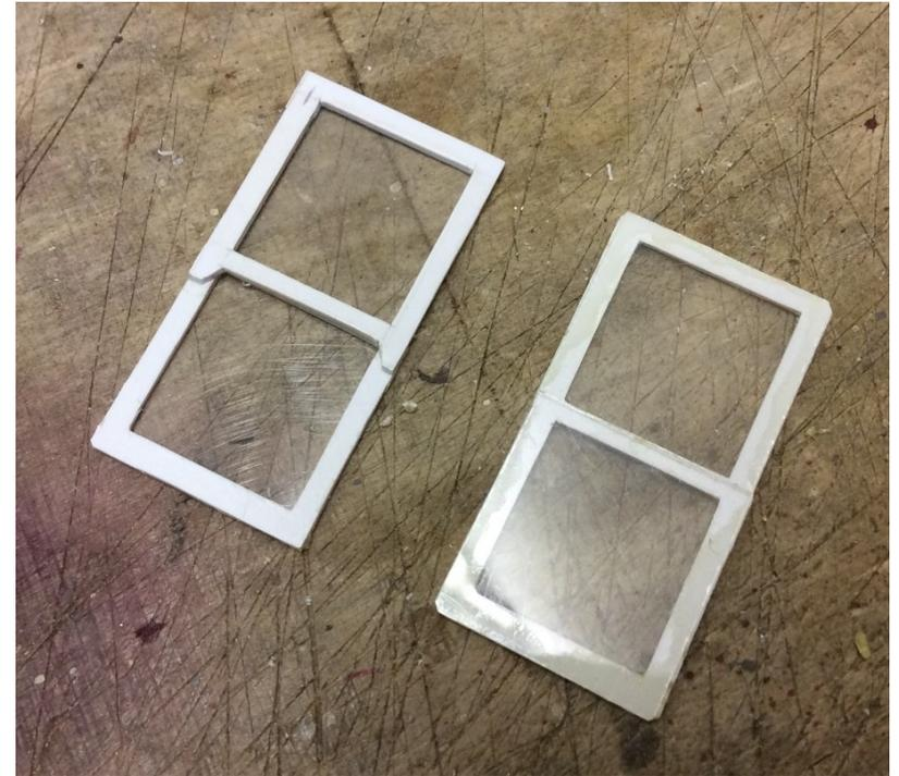
Slaters Plastiglaz (Ref:0312) was used throughout the building. With minute spots and smears of Super-glue on the insides of the windows, the oversize glazing pieces were placed in position. Each glazing piece was then cut flush. Wherever glue seeped outside the sashes, the glazing was quickly removed then replaced with new glazing.
