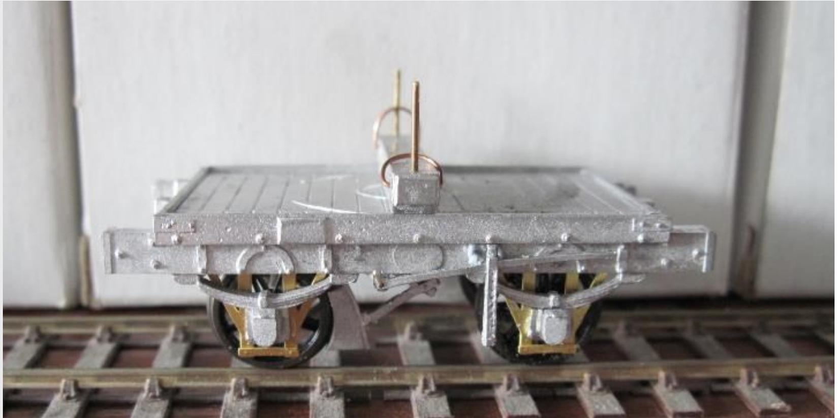
The cast parts for the brakes need some work. The lever supplied by Chris is marginally long, so I cut it and redrilled a hole for the pivot.
